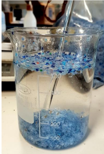
Figure 36. Flakes separated by density
