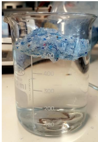
Figure 35. All the material floating at the beginning of the pre-washing
