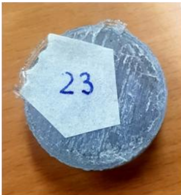
Figure 84. Printing with filament referenced to test number 23 (Scenario 3.2 AEV 331)
