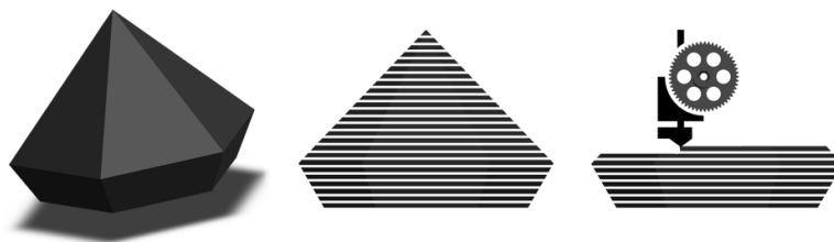
Figure 11 - Schematic representation of the printing of an object by layers (Emaze)
