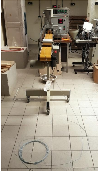
Figure 67. General view of AEV 331 extruder
