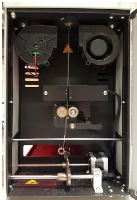
Figure 39. Extrusion with 3Devo-composer 450 using virgin PET
