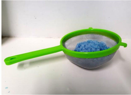
Figure 38. Decanted flakes between the steps of the washing process
