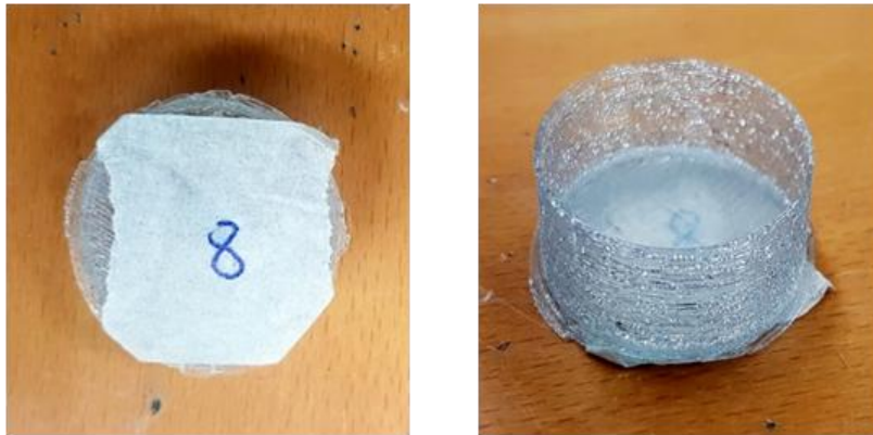
Figure 79. Printing with filament referenced to test number 8 (Scenario 3.1 3Devo)
