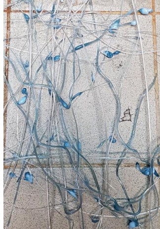
Figure 42. Discarded filaments due to clogging problem
