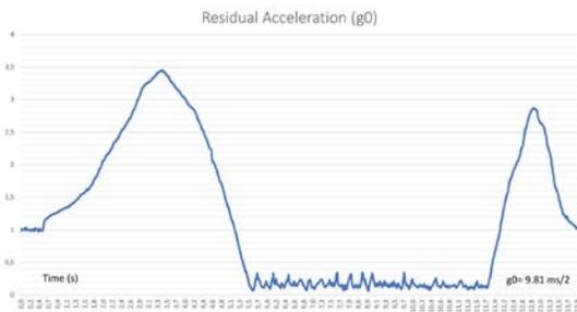
Figure 3: Residual acceleration of a parabola conducted with the CAP10B aircraft in this research.
