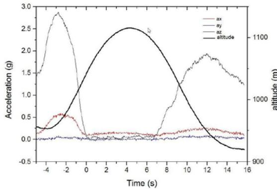
Figure 2: Flight profile of an average parabola performed during the research flight.
