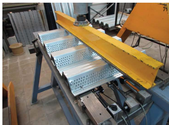
Fig. 10. Load spreading system. Internal support test.
