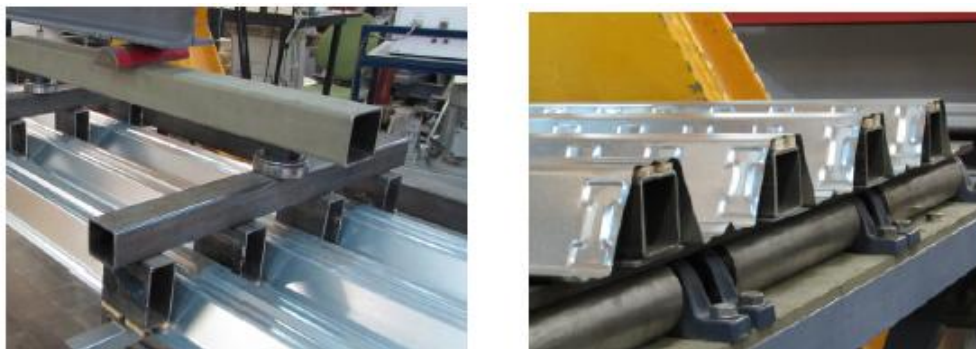
Fig. 5. Loading system detail with W60-Plain profile (left) and support detail with W60-Emb profile (right).
