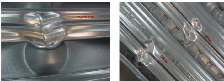
Fig. 11. Local buckling (M+): a) W60-MD-0.75 b) W60-MD 1.00 c) W60-MD-1.20 d) W60-Plain-0.75 and W60-Emb-0.75
