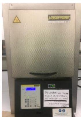
Figure 3.10: Furnace where the printed specimens were sintered.
