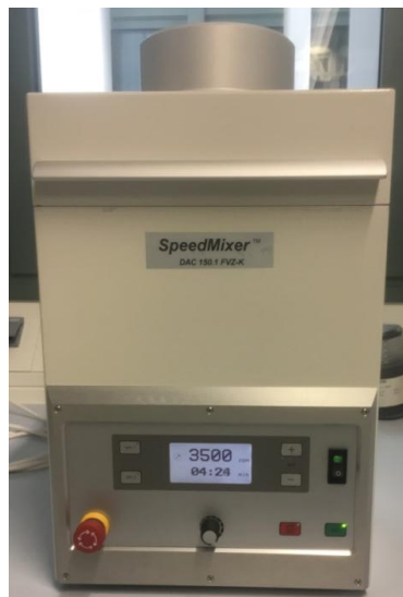
Figure 3.4: SpeedMixer, the machine used to mix the hydrogel and ceramic pastes.
