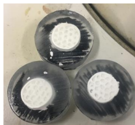
Figure 3.12: Hexagonal samples put inside the resin to polish them.
