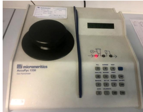
Figure 3.16: Helium pycnometer used during the Bachelor's project, to measure the density of samples 13 and 14.
