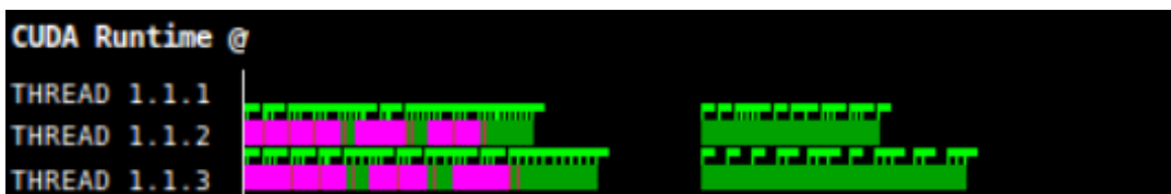
FIGURE 4.4: Data transfer between the host and the GPUs. The pink color represents data transfer from the host to the devices, the green represents transfers from the devices to the host.
