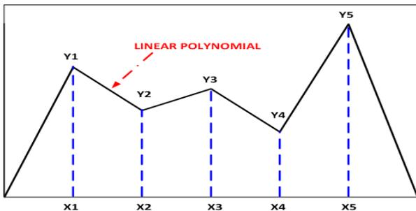
Figure 1. Example of interpolation with linear splines.
