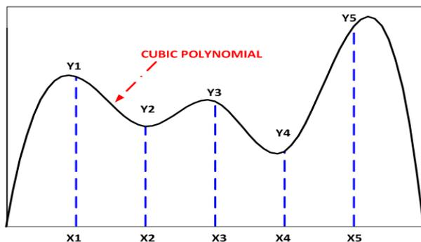
Figure 2. Example of interpolation with cubic splines.
