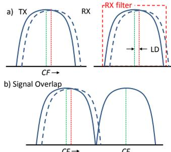
Fig. 2. Signal misalignment and overlap
