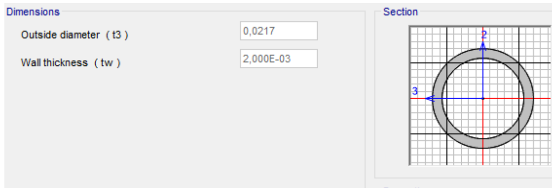
Picture 26. Geometry of the new bracings
