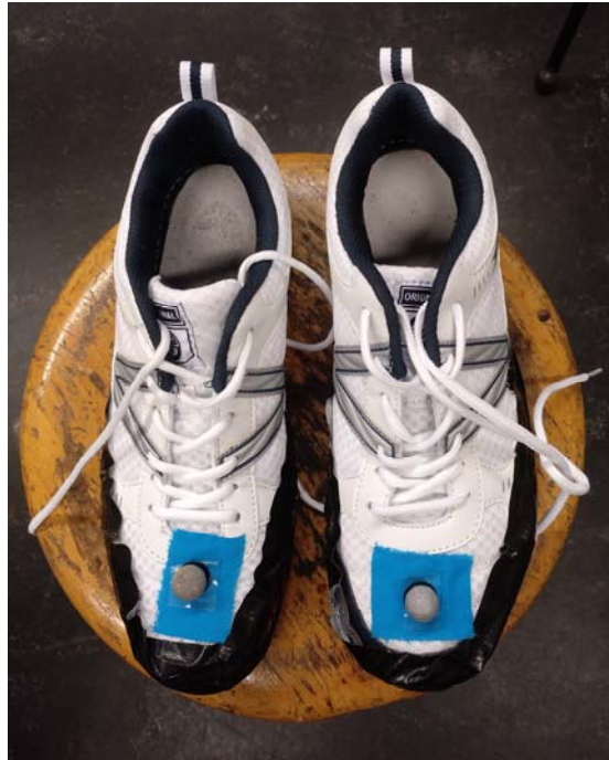
Figure 9 — Victory shoes used in the experiment. Left shoe is the control condition (N) and right weighted shoe of 315 grams (C). It is not possible to recognise visually the different weight.
