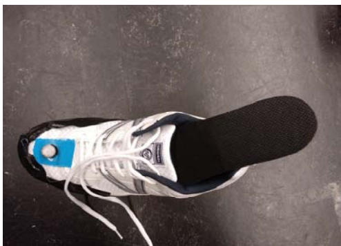
Figure 12 — Right way of introducing the Moticon insole.
