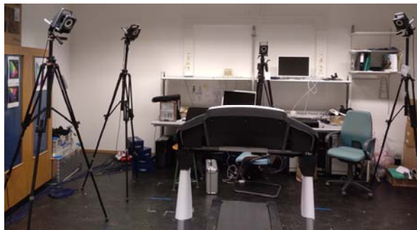
Figure 6 —Treadmill and Vicon camera's disposition for the experiment
