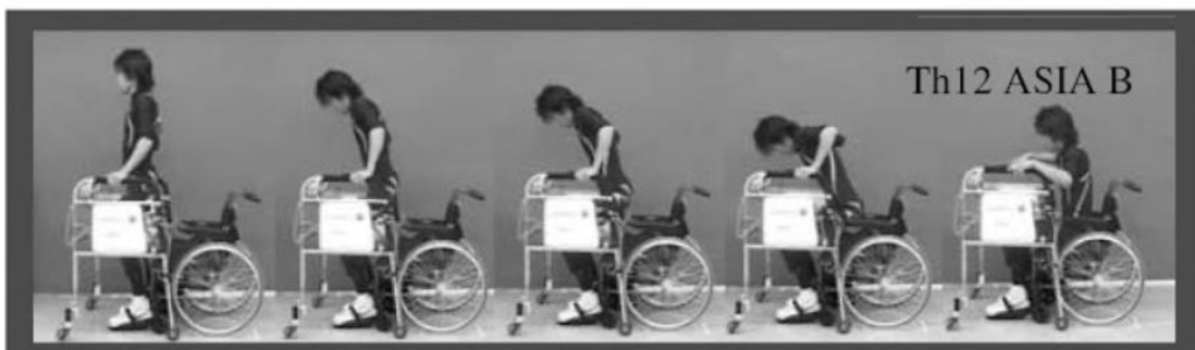
Figure 1.2 Subject with the WPAL executing the Sit-to-Stand motion [22]
