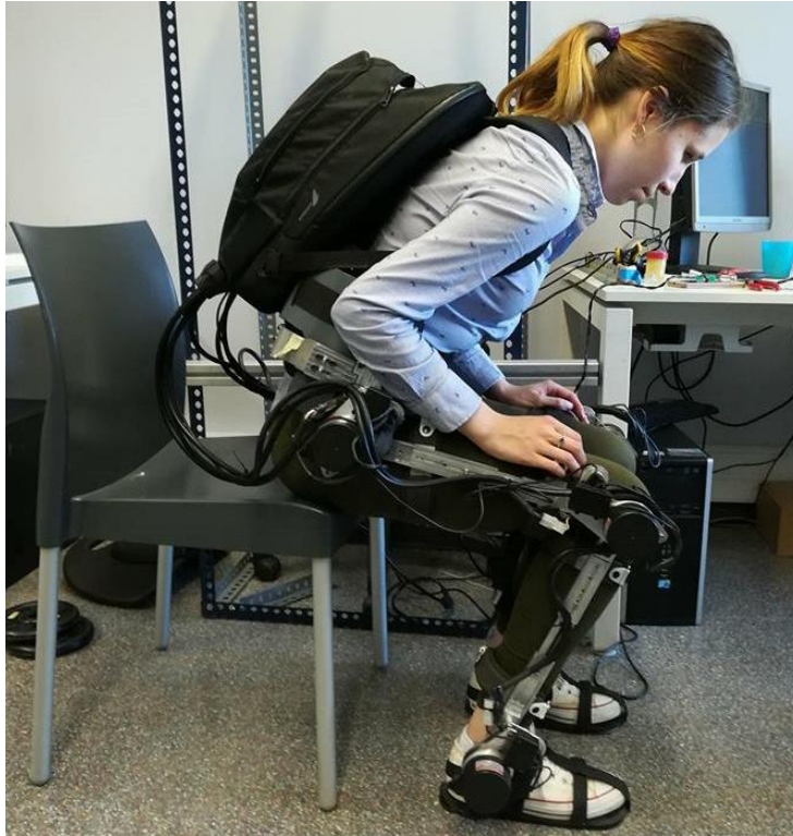
Figure 2.12 Initial position required to activate the movement of exoskeleton
