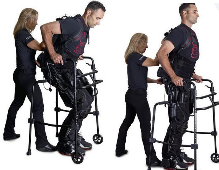
Figure 1.3 Subject with the eLEGS during an evaluation [24]
