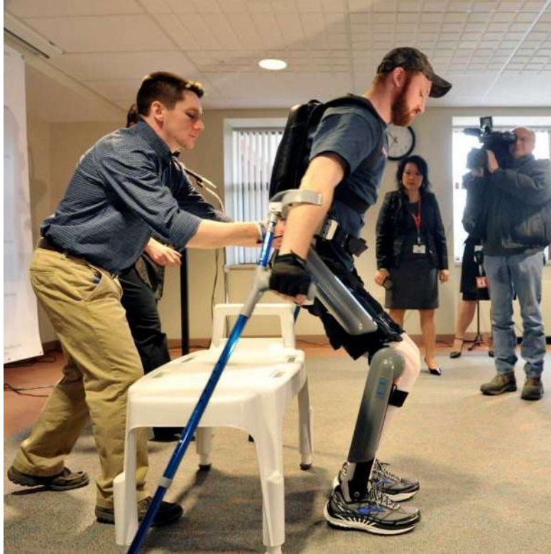
Figure 1.4 Patient rises with the ReWalk Rehabilitation Version [26]
