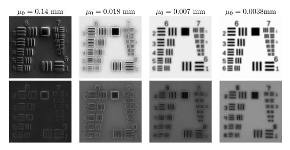
**Figure 3.** Upper row: simulations using the GPU algorithm for different degrees of coherence. Lower row: experimental results for the same degrees of coherence.
