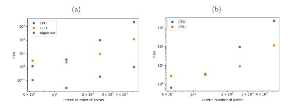
**Figure 2.** Execution times of the CPU, GPU and algebraic implementations. (a) correspond to the simulations with constant Fourier Transform of the complex degree of coherence and (b) are those with constant complex degree of coherence. (b) does not show the algebraic implementation as it was not able to finish due to memory constraints.
