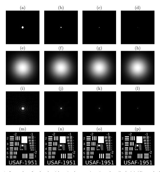
**Figure 1.** Input data for the algorithms in the two situations described. (a)-(d) are the Fourier Transforms of the complex degree of coherence for the first case, (e)-(h) are the complex degrees of coherence for the second case, (i)-(l) are the PSFs for both simulations and (m)-(p) are the object amplitudes.
