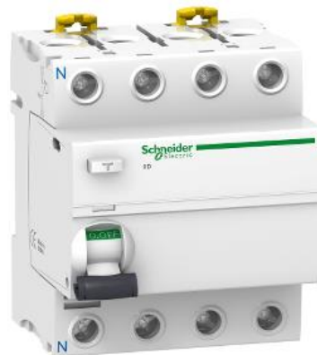
Figure 8.29- A9R21463 differential switch of 63 A, 30 mA sensitivity, 4 poles. Source [46].
