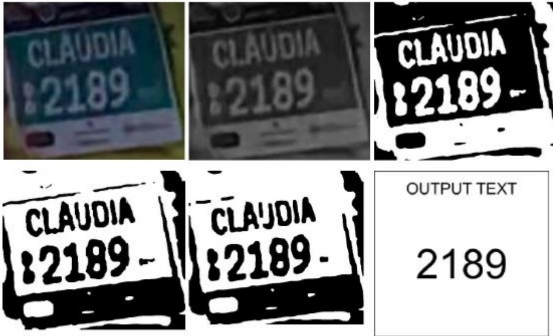
Figure 4.6 – Dorsal with a correct number read by OCR
