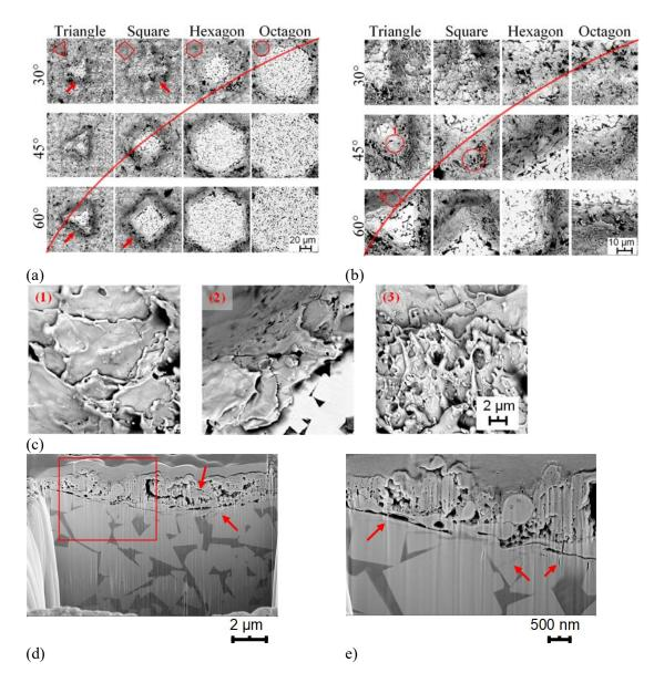
**Figure 6.** Shape and morphological characterization of single pyramids at **(a)** large and **(b)** small scale, **(c)** high magnification details of selected positions, **(d)** cross-sectional analysis by FIB at the bottom position, and **(e)** close-up on the melting zone.
