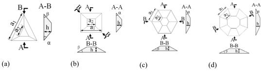
$a_1$ : bottom side length,  $a_2$ : top side length h: pyramid height,  $\alpha$ : slope at the measuring position A-A (side angle),  $\beta$ : slope at the measuring position B-B
