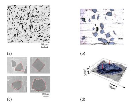
Figure 1. Microstructural and geometry aspect of (a) 10CoC hardmetal grade, (b) conventional honing stone, (c) typical grain shapes (triangle, square, hexagon and octagon), and (d) one single abrasive grain.
