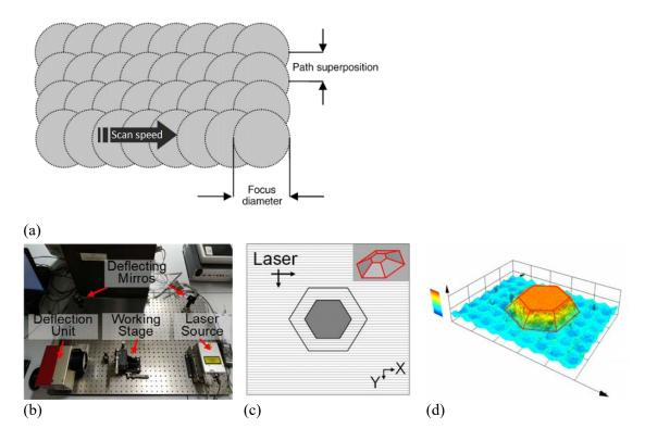
Figure 3. (a) Schematic illustration of the laser machinig parameters, (b) composition of laser set-up, (c) laser beam path, and (d) reconstructed 3D model based on the dimensional measurements by LSM.
