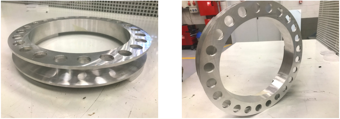
Figure 4.3: Support for the prototype of one coil.
