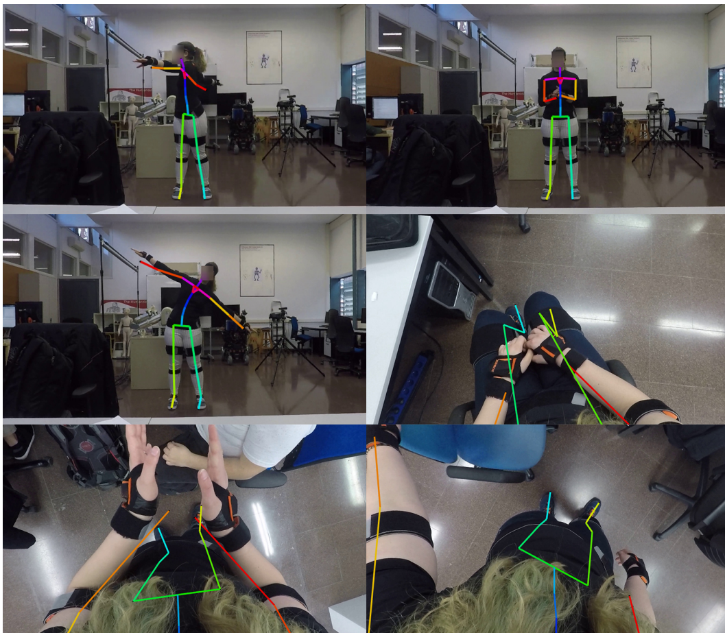
Figure 3.6: Projections of MVN Awinda data onto a video
