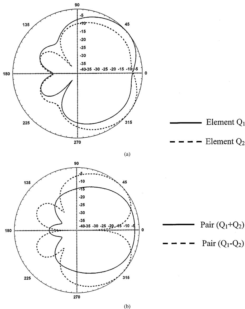
Fig. 15. Reconfigurable radiation pattern for the MEMS switch-tunable *qdime* antenna. (a) Copolar  $x-z$  plane patterns corresponding to the *qdime* elements  $Q_1$  and  $Q_2$ . (b) Copolar  $x-y$  plane patterns corresponding to the pair *qdime* element-combination  $(Q_1 + Q_2)$  and  $(Q_1 - Q_2)$ .
