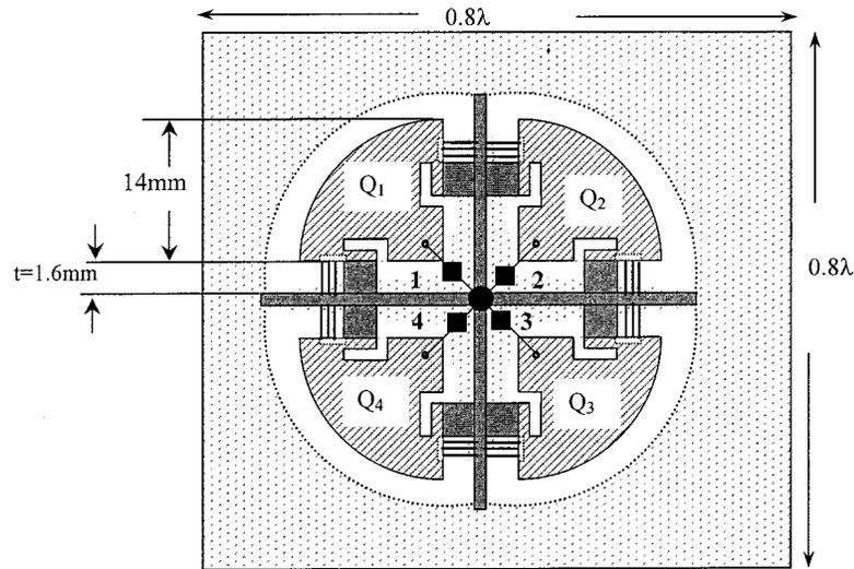
Fig. 12. Top view of the lower-patch plane of the MEMS switch-tunable four-element *qdime* antenna configuration.  $Q_1, Q_2, Q_3, Q_4$ : *qdime* antennas. 1, 2, 3, 4: MEMS switches. ( $w_u = 5$  mm,  $w_l = 4$  mm,  $l_s = 5.9$  mm,  $h_u = h_l = 1.6$  mm,  $S = 22$  mm).
