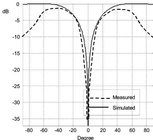
Fig. 7. Simulated (solid line) and measured (dashed line) radiation pattern at 985 MHz for the  $TM_{01}$  Mode of the designed antenna.
