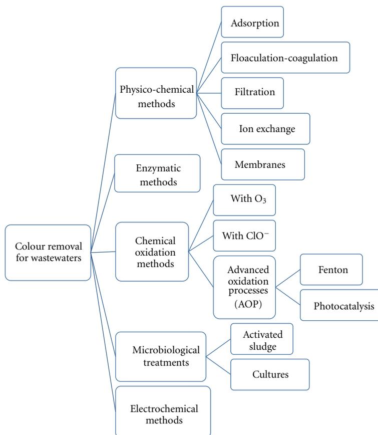
FIGURE 5: Methods for textile wastewater color removal.
