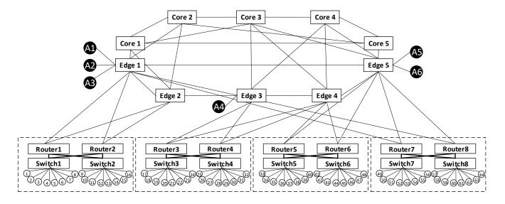
Figure 2: As in [15], Physical network of four datacenters located in separate geographical areas.
