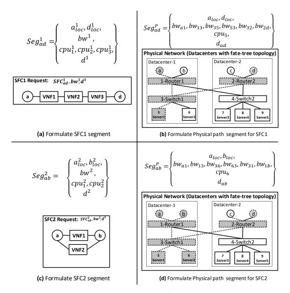
Figure 1: Segments' formulation demonstration: (a) shows the service function chain  $SFC_{ad}^1$  and its segment, (b) shows physical network and the segment of a candidate hosting path  $P_{ad}$ , (c) shows service function chain  $SFC_{ab}^2$  and its segment, (d) shows physical network and the segment of a candidate hosting path  $P_{ab}$
