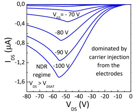
Figure 3. Output characteristics of the picene-based TFT. NDR effect is observed for  $V_{DS}$  voltages higher than  $V_{DSAT}$
