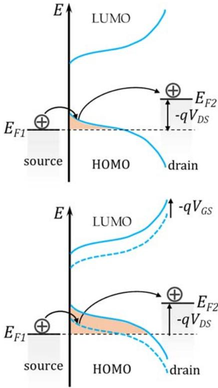
Figure 4. (Top) Schematic representation of the energy levels of the source, drain and DOS of the p-type picene TFT. (Bottom) Application of negative  $V_{GS}$  voltage shifts down the picene DOS, increasing the number of available states.
