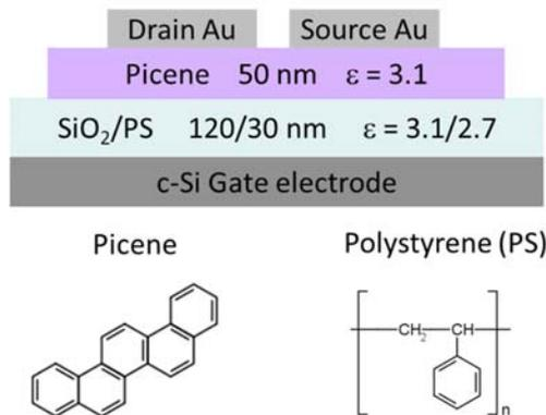
Figure 1 (Top) Scheme of the fabricated TFT based on picene. Thicknesses and permittivity values of the picene and dielectric layer are showed. (Bottom) Chemical structure of the picene and polystyrene molecule.
