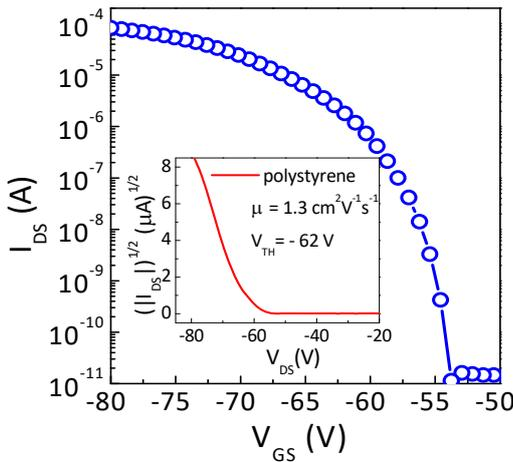
Figure 2. Transfer characteristics. (Inset) Saturation characteristics, from which the field-effect mobility and Threshold voltage are estimated
