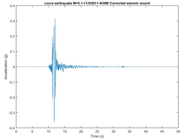
Fig. 1. The nort-30-west component of the LOR accelerogram obtained in the 2011 Lorca (Spain) earthquake. This seismic record was processed by Seismograms Analyzer-e software. [1].
