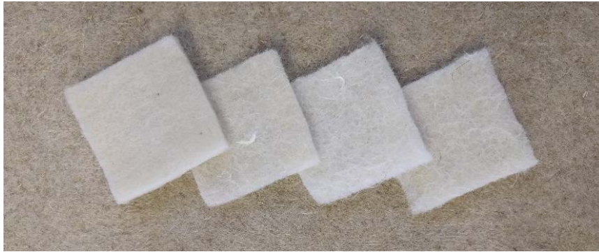
Figure 1A. Appearance of needle punched samples. From left to right: CFs0W100, CFs10W90, CFs25W75 and CFs50W50.
