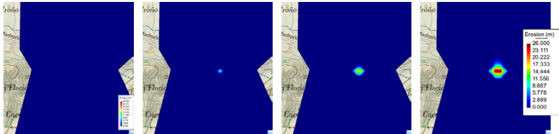
Figure 74. Smooth contour fill representation of the erosion. From left to right, erosion at times 1200 s, 2400 s, 3600 s and 4800 s.
