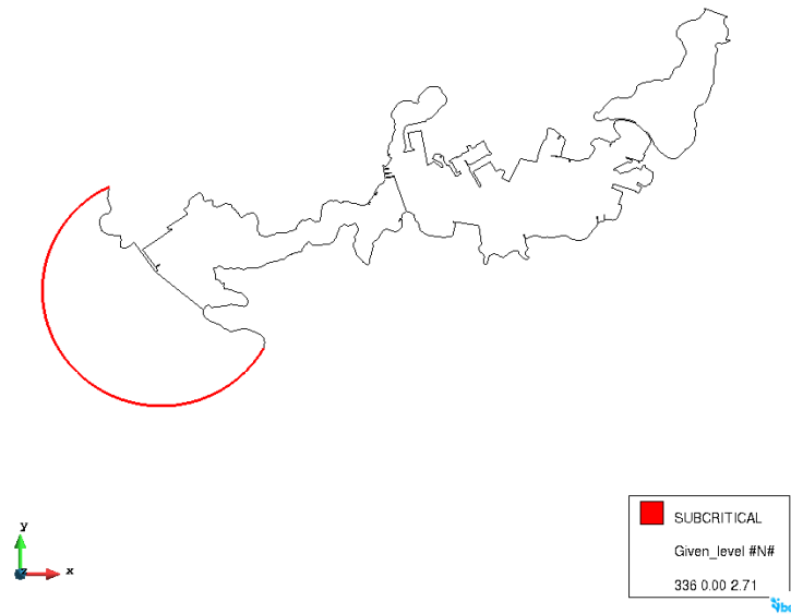
Figure 131. Location of the open boundary of the model.
