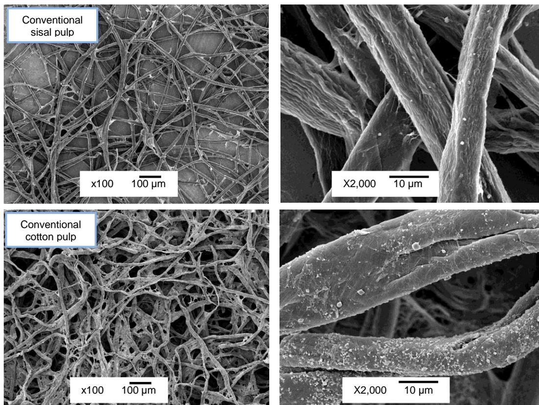
**Fig. 1.** SEM images at different magnification of conventional sisal pulp (1<sup>st</sup> row) and cotton linters (2<sup>nd</sup> row)
