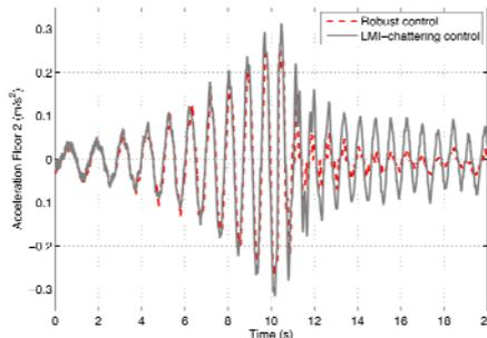
Figure 6. Floor 2 acceleration using (6) and (7) controls, when sensor fault appears.
