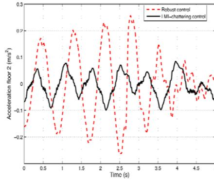
Figure 2: Acceleration of Floor 2 using robust control versus chattering-LMI control.
