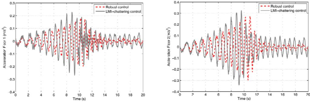
Figure 4. Accelerations of Floor 1 and 2 using robust control (6) versus LMI-chattering control (7), when structural fault appears.
