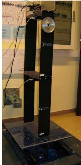
Figure 3. Shake Table II with a hardware-simulated structure fault.
