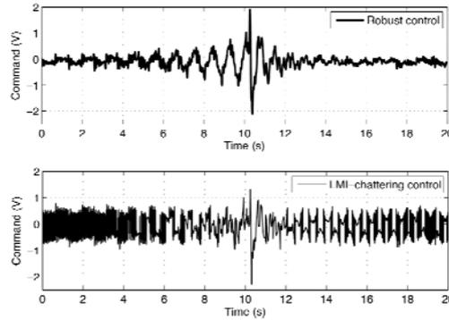
Figure 7. Signal from robust control (6) and LMI-chattering control (7), when sensor fault appears.
