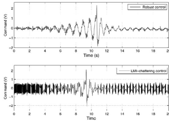
Figure 5. Robust control (6) versus LMI-chattering control (7), when structural fault appears.
