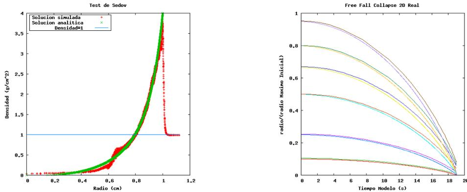
Figure 1: *Left*: Sedov test, density profile with across time  $t = 2.16 \times 10^{-2}$  s. *Right*: Collapse of a cylinder of infinite height. It represents the simulated evolution with ISFAA and the theoretical trajectory, beginning with different initial radii.
