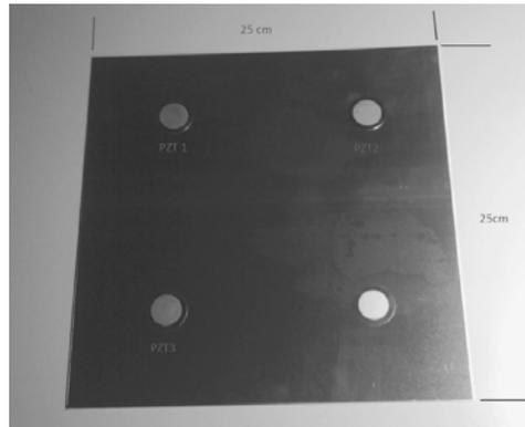
Figure 1: Aluminium plate: Dimensions and PZT's location.
