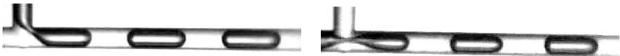
Fig 1: example of bubbles being generated with both methods with the same conditions of gas and liquid injection.
