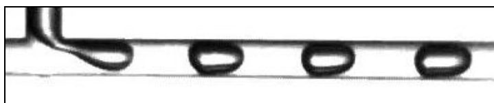
Figure 1: Detail of the bubble generator. Gas is injected from the top and liquid from the left side.
