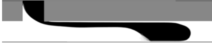
Figure 8: Gas thread generation without squeezing. U_{SL}=0.318 m/s and U_{SG}=0.182 m/s.
