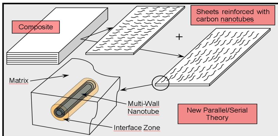
**Figure 2:** Representation of formation for reinforced composite.
