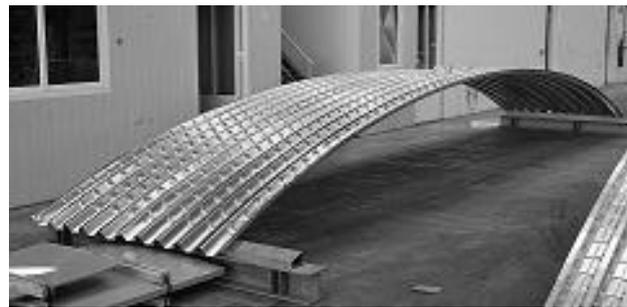
*Fig. 2. Arch manufactured from a ribbed sheet.*
