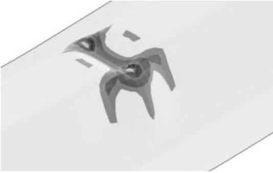
Fig. 7. Plastic strains in a sheet without corrugations after limit point.
