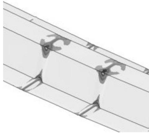
Fig. 8. Plastic strains in a sheet with corrugations after limit point.
