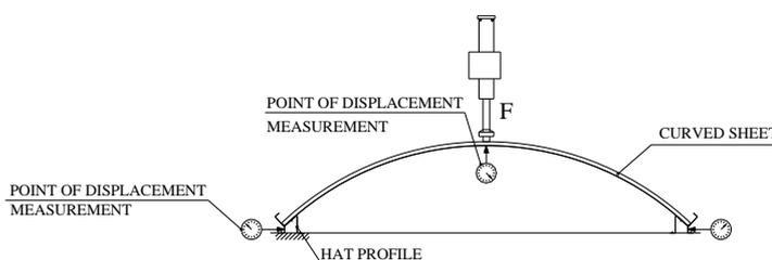
*Fig. 4.* Test arrangement.
