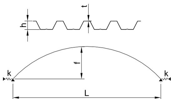
*Fig. 3.* Geometric parameters of the sheet.
