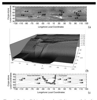
Figure 6. Erosion (light) and accretion (dark) patterns during the field experiments (a) and Breached bar and a well developed rip channel over which the lagrangian buoys drifted (b)
