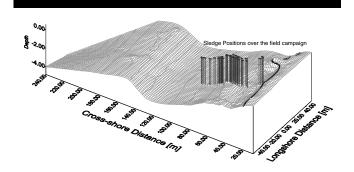
Figure 2. Sledge positions during the Delta'96 experiments and initial bathymetry (in local coordinates).
