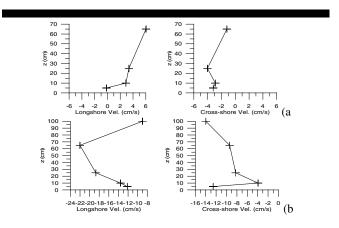
Figure 4. Longshore and cross-shore velocities, tests 0503 (low wave-energy) and 0509 (high wave-energy conditions).
