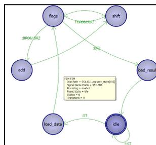
**Figure 7** Multiplier's control unit state diagram ([Ctrl+Click to follow the link of the picture in normal size \[p\]](#)).
