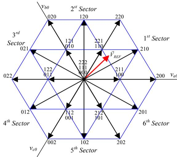
Fig. 3: Space-vector diagram of the NPC converter
