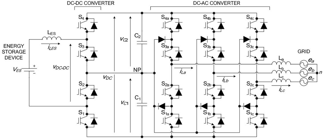
Fig. 1: 3L DC-DC and NPC DC-AC Converter
