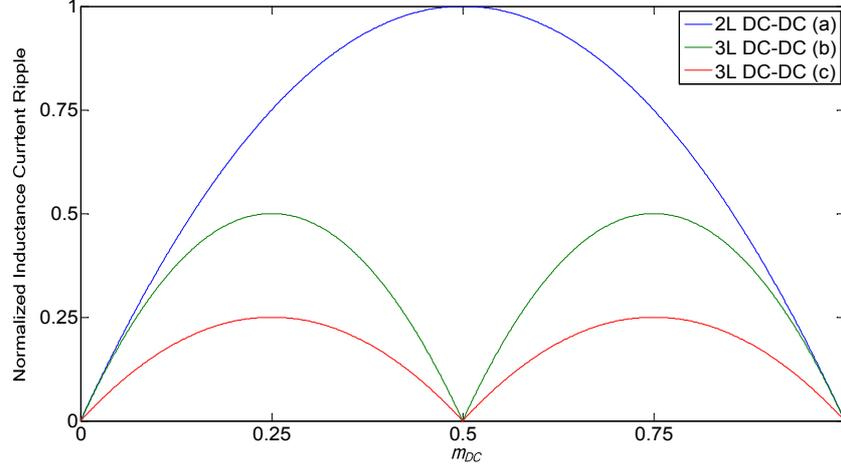
Fig. 2: Normalized inductance current ripple in (a) a 2L DC-DC converter and in a 3L one with (b) the same, and (c) double switching events
