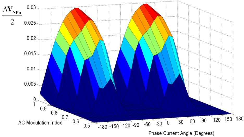
Fig. 7: Normalized NP voltage ripple in worst case
