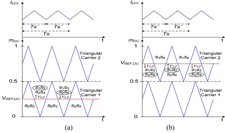
Fig. 4: PWM modulation for NP voltage balance when (a)  $m_{DC} < 0.5$  and (b)  $m_{DC} > 0.5$
