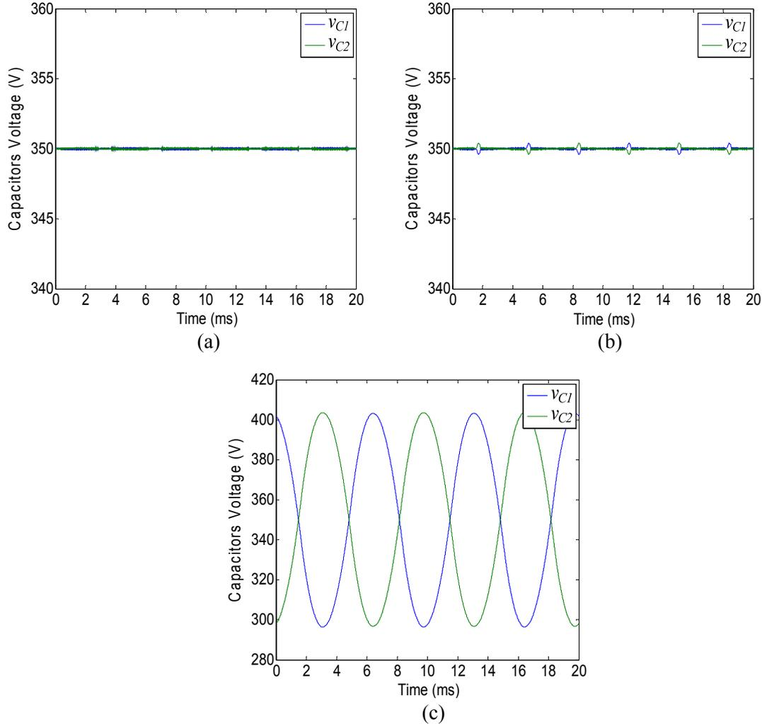
Fig. 6: DC-link capacitors voltage for the case  $I_{RMS} = 100$  A,  $f = 50$  Hz,  $m_{AC} = 1$  and  $\varphi = -60^\circ$  with: (a)  $m_{DC} = 0.5$ , (b)  $m_{DC} = 0.6$  including a 3L DC-DC converter in the topology, and (c)  $m_{DC} = 0.6$  without a 3L DC-DC converter
