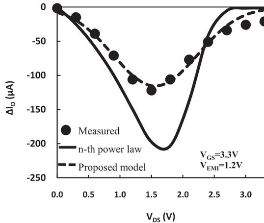
Fig. 3 Drain current shift due to EMI.
