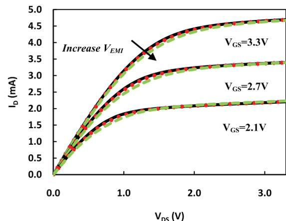
Fig. 2 Experimental  $I_D$ - $V_{DS}$  characteristics under EMI conditions. Continuous lines correspond to MOSFET without EMI and dot and dashed lines correspond to  $I_D$ - $V_{DS}$  under EMI of 0.6 V and 1.2 V, respectively. Curves for  $V_{GS} = 3.3\ \text{V}$ , 2.7 V and 2.1 V are shown.
