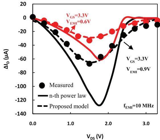
Fig. 5 Validation of the proposed model under different EMI amplitude.
