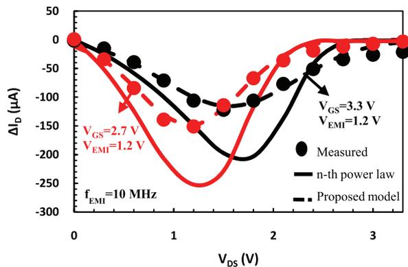
Fig. 6 Validation of the proposed model under different  $V_{GS}$  conditions.
