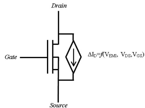
Fig. 4 Proposed MOSFET model under EMI conditions.
