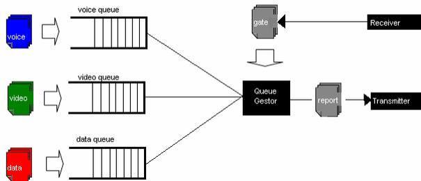
Figure 3. ONU functional schema
