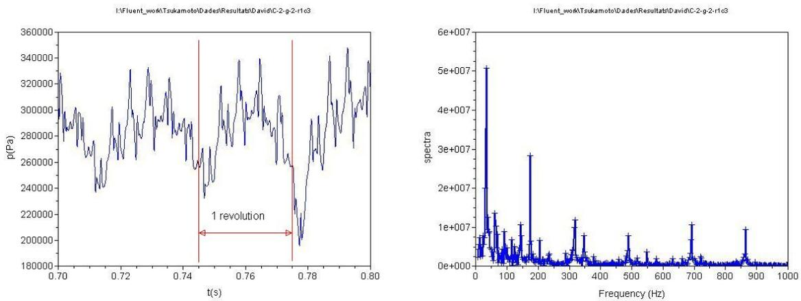
Figures 5, 6 and 7 show in detail the pressure fluctuations at point r1c3 and its correspondent  $Z_iN$  frequencies (after treating the obtained pressure data with a Fourier transform) for 3 different turbulence models: Spalart-Allmaras, Realizable  $k-\varepsilon$  and SST  $k-\omega$ .
