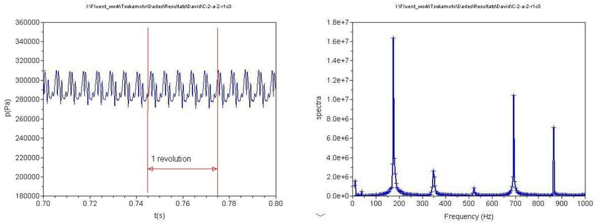
**Figure 6:** Realizable  $k-\epsilon$  model. Left: calculated unsteady pressure at point r1c3; right: frequency domain.
