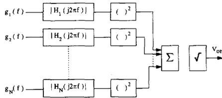
Fig. 2. Model for calculating the output noise of a general linear circuit: each noise source contributes according to its particular transfer function.
