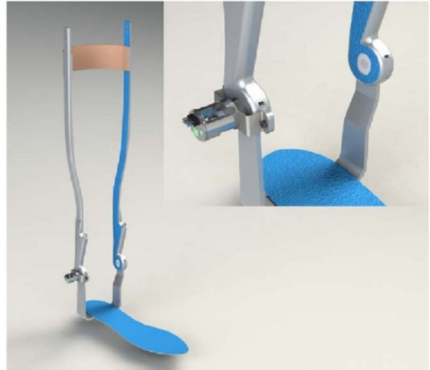
FIGURE 6. Ankle module with a detail of the encoder
