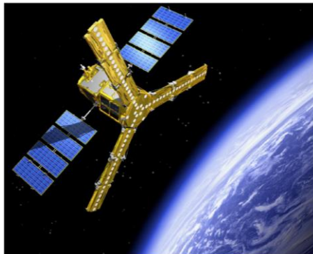
Figure 1.1 View of SMOS satellite. The SAR called MIRAS for Microwave Radiometer with Aperture Synthesis, is composed by 69 antennas on a Y shaped deployable platform.
