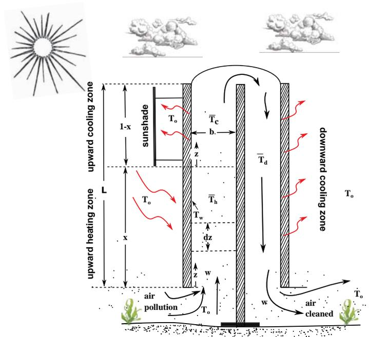
FIG. 2: Schematic of flow in the vertical solar plate.
