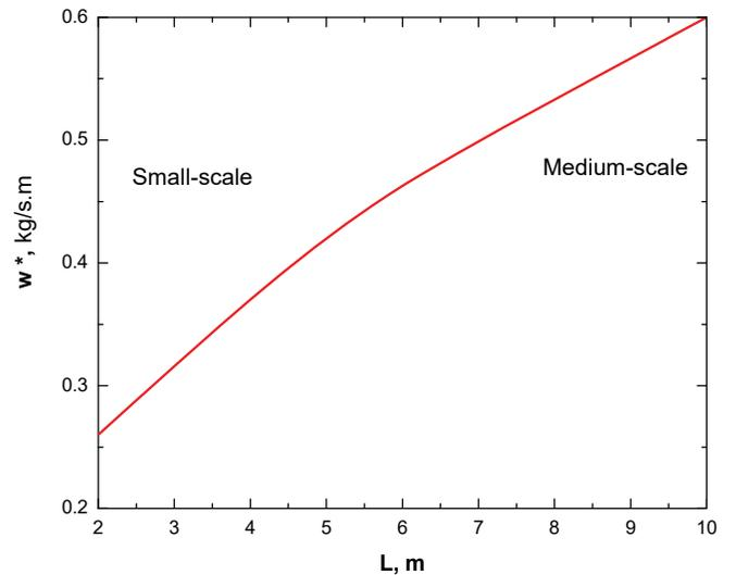
FIG. 4: The attainable air flow rate per unit width and as function of the height  $L$  and using  $x = 1$ .
