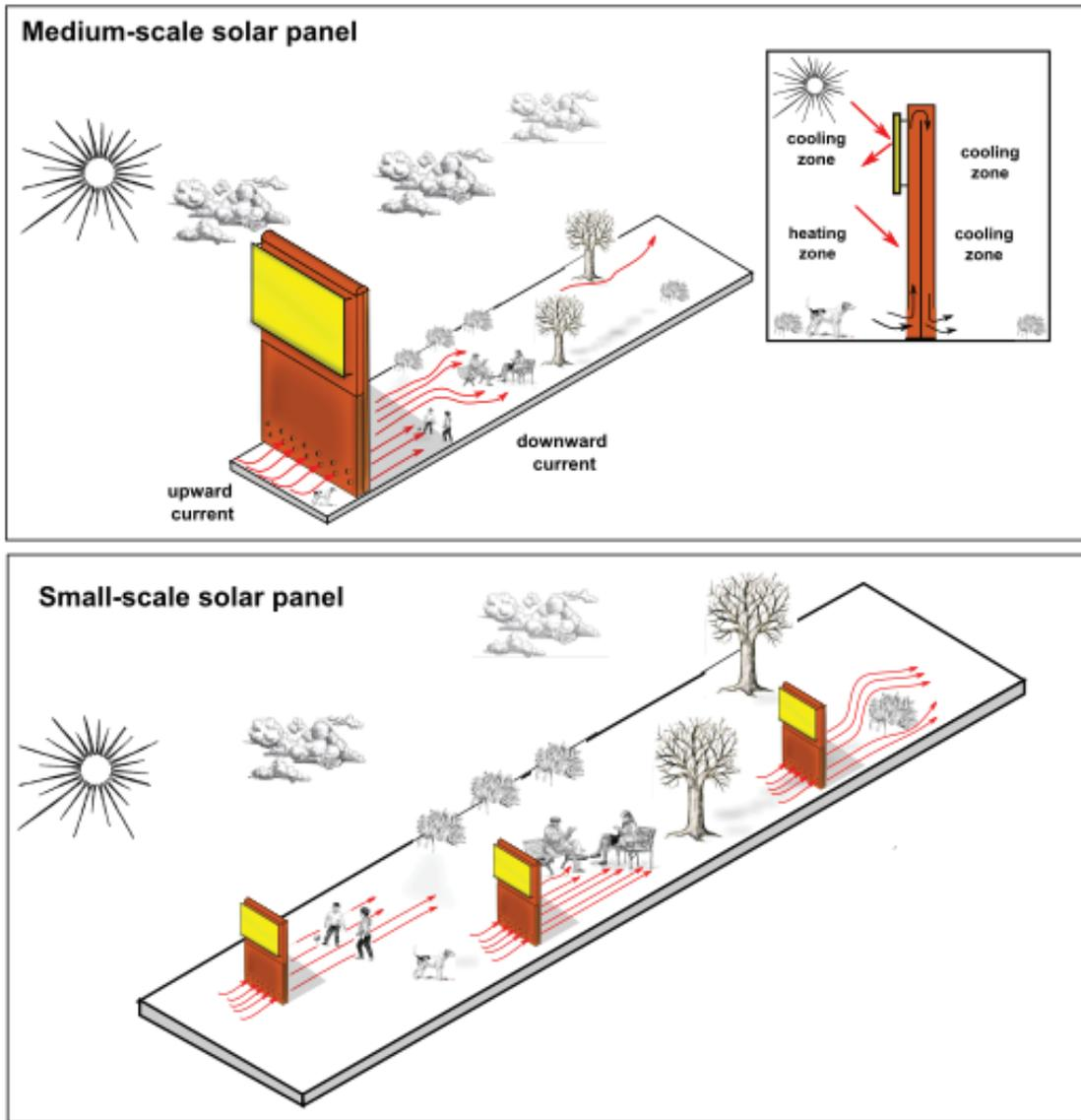
FIG. 1: A pictorial scheme of the idea discussed. At the top a 10 meters panel for local medium-scale air cleaning, at the bottom, a 2 m panel for local small-scale
