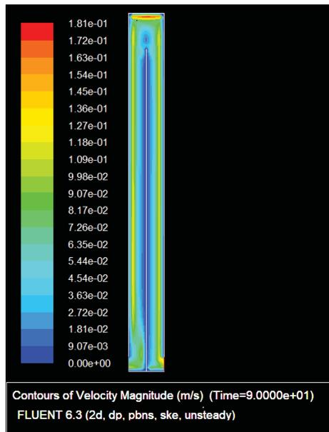
FIG. 6: Velocity profile from the CFD simulation for a 1-m-height column.
