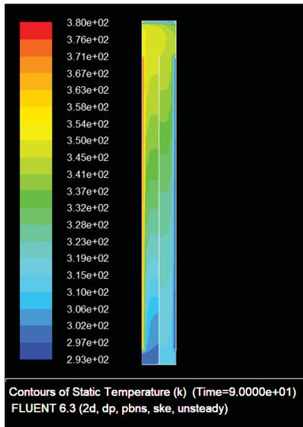
FIG. 5: Temperature profile from the CFD simulation for a 1-m-height column.
