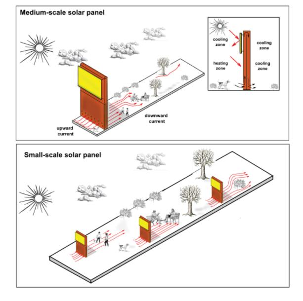
FIG. 1: A pictorial scheme of the idea discussed. At the top a 10 meters panel for local medium-scale air cleaning, at the bottom, a 2 m panel for local small-scale
