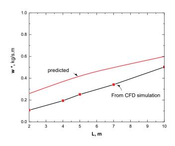
FIG. 7: Comparison between the predicted air flow rate per unit width and the CFD simulation.
