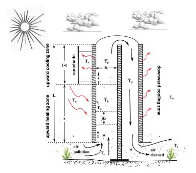
FIG. 2: Schematic of flow in the vertical solar plate.
