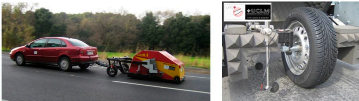
Figure 3. Tiresonic Mk4-LA 2 IC for acoustics characterization of road surfaces and detail of the microphone positions.
