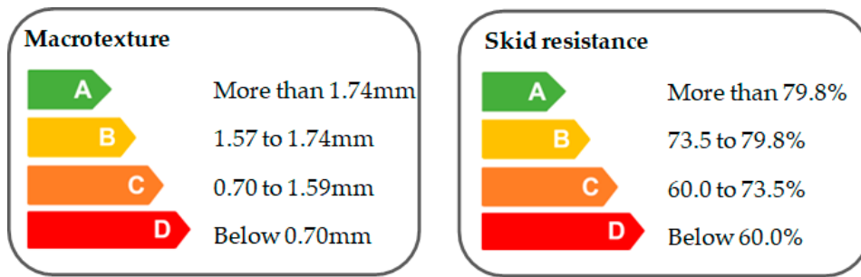
Figure 21. Macrotexture and skid resistance global label.
