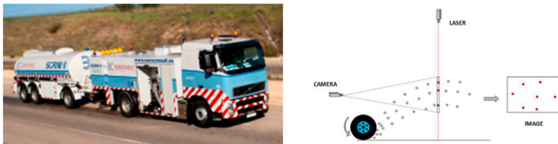
Figure 2. Splash and spray trailer and measuring details.
