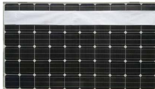
Figure 5. Photo of module Tenesol 2200 with shadows 22-03-2018
