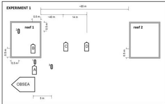
Fig. 2. Set-up experiment one
