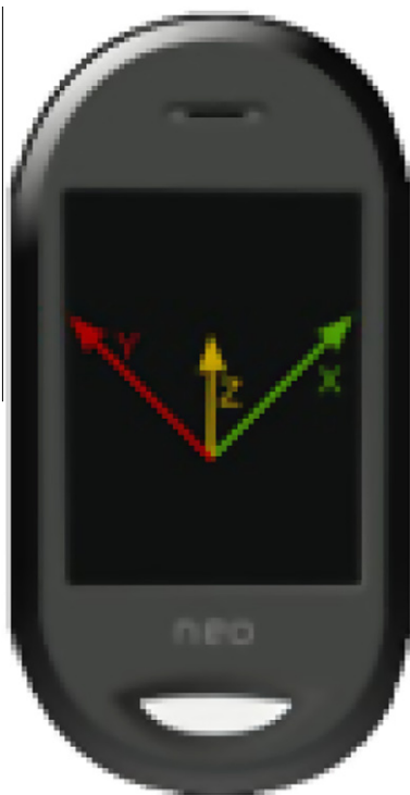
Fig. 4. Orientation of the axes in the Openmoko Neo FreeRunner accelerometer used.
