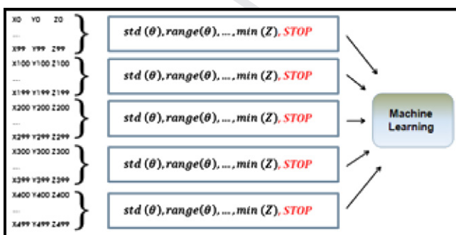
Fig. 2. Features calculation sample for stopping (or walking) activity.
