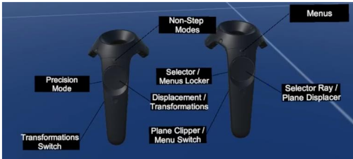
Figure 34 Scene capture of the controller's prefab tooltips
