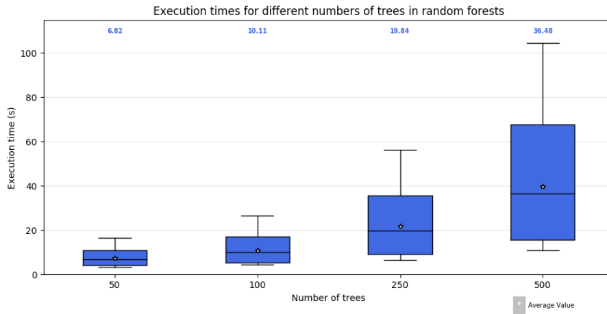
FIGURE 5.8: Boxplot of the execution time of random forests for different number of trees.
