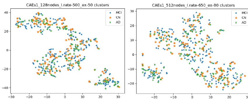
Figure 4.3: Manifold visualization of reduced data by CAE with 2D slices 1. Data was compressed into 128 nodes (left) and 512 nodes (right). On the left there is the representation of the data when reduced into 128 nodes and visualized using t-SNE parameters: learning rate = 500 and early exaggeration = 50. On the right we can see the representation of the data when reduced into 512 nodes and visualized with t-SNE parameters: learning rate = 650 and early exaggeration = 80.
